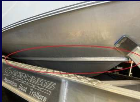
Planing Strakes (aid lift and deflect spray)
